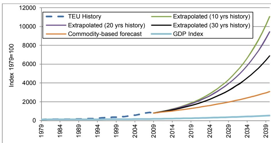
The extrapolated forecasts would create a potential over-estimation of required port capacity for container handling by 300% for the 20-year extrapolation, compared with the commodity-based forecast. This shows the potential danger of planning and investing in infrastructure on the basis of extrapolating historic trends for containers.
